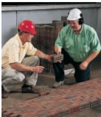
To maintain color uniformity throughout the four-year span of brickmaking, brick from each production run was laid in a representative panel and then compared to the master panel established for color reference at the start of the Sprint project.
